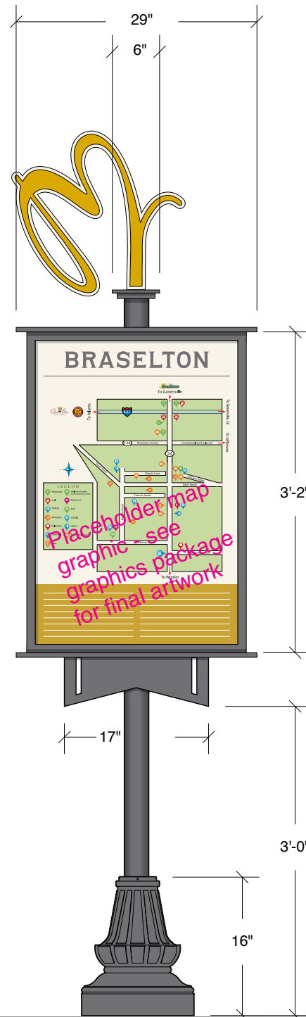
3 E. Pedestrian Kiosk - Back Elevation SCALE: 3/4" = 1'-0"
